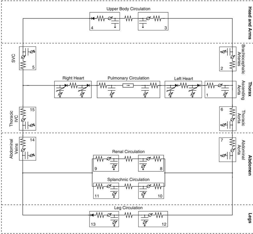
**Fig. 2.1** Circuit representation of the hemodynamic system. *IVC*: inferior vena cava; *SVC*: superior vena cava
