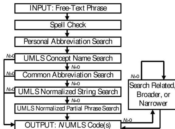
Figure 1. A flow chart of the search process, where  $N$  is the number of UMLS codes found by the algorithm.
